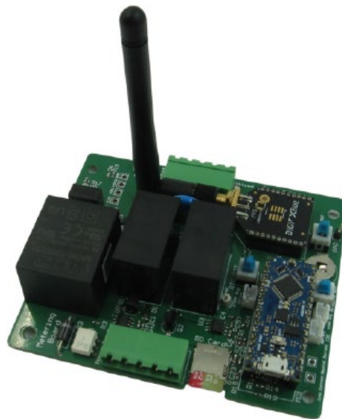
Figure 1. Smart Metering Prototype
